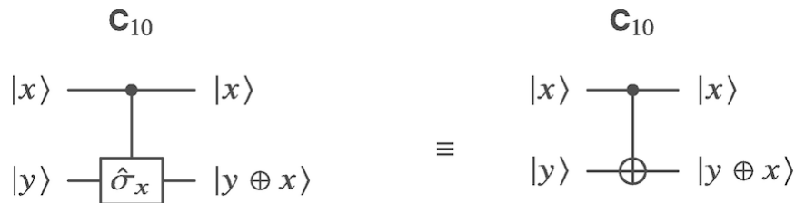
Fig. 3.4 Two equivalent circuits representing the action of the CNOT gate \mathbf{C}_{10} . The filled circle is placed on the control qubit wire, while the XOR symbol \oplus recall the action of the gate on the target qubit
